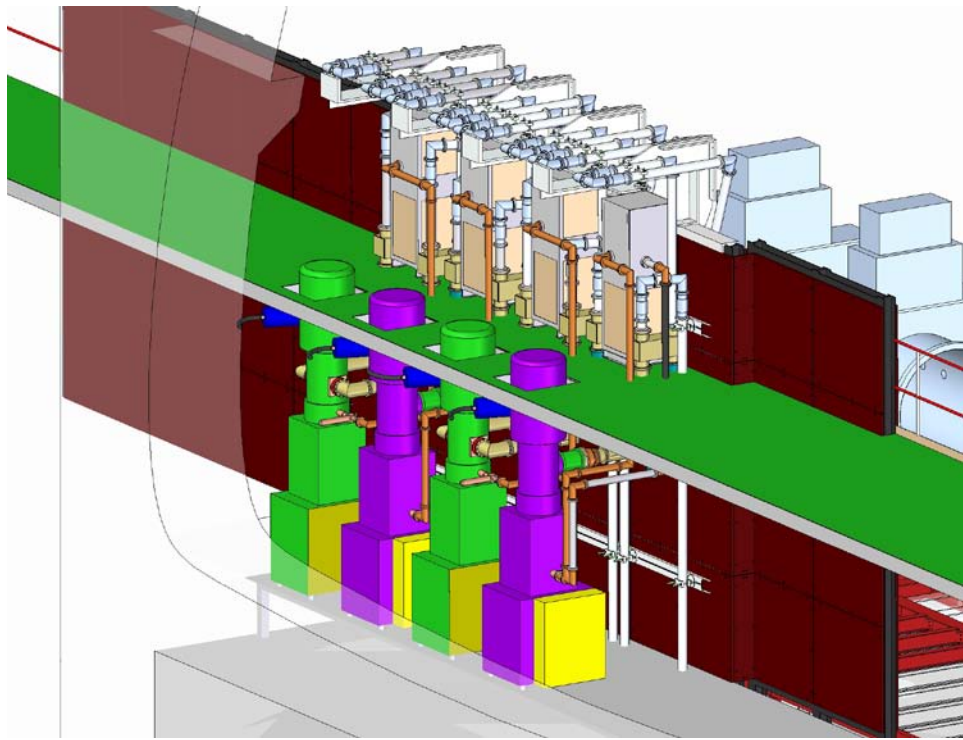
Fig 5: layout of amplifiers and coax system behind shield wall
