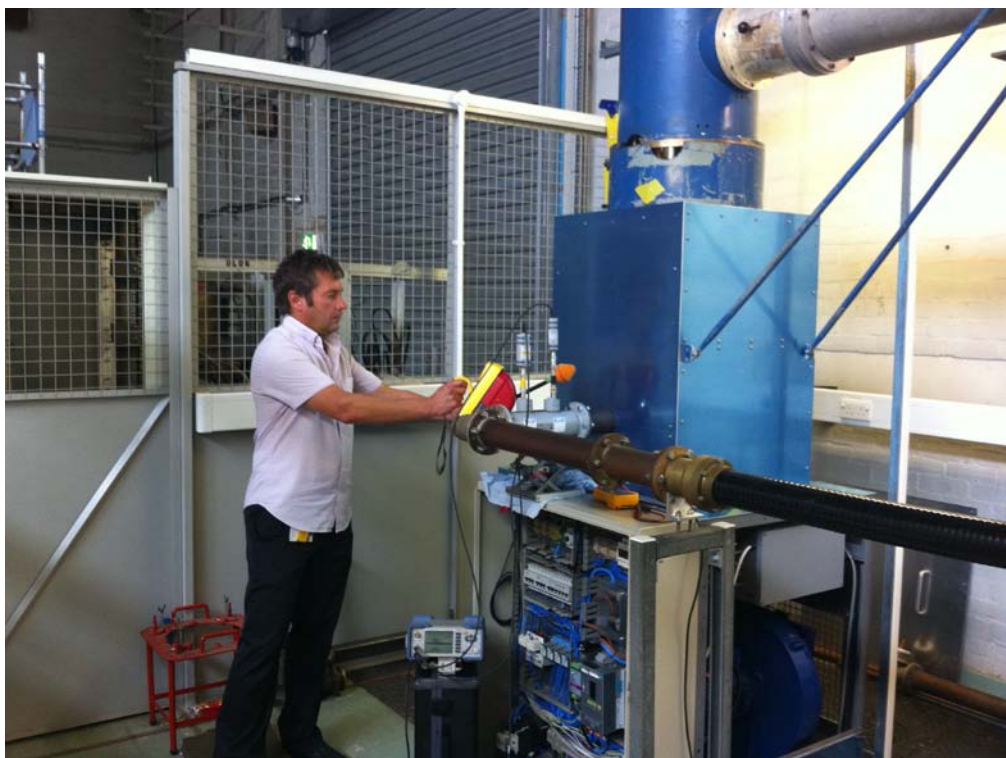
Fig 1: 116 amplifier operating at 1MW, no x-rays or microwave radiation detected
