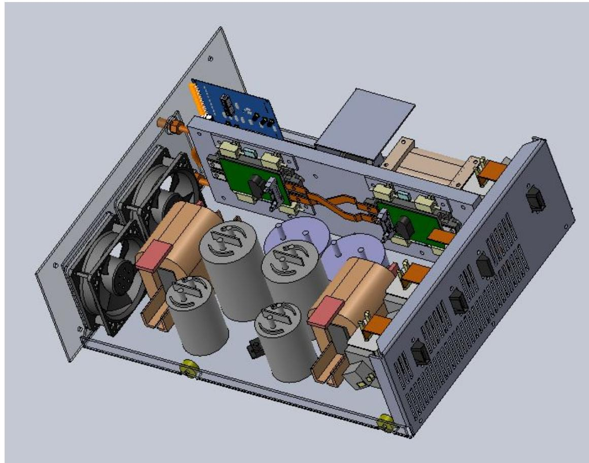
Using the same case and heat sink, we have rearranged all new components. the new output stage passive filter with high current snubber capacitors is displayed in the central part
