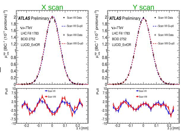
Gauss+p0 fit quality suffers in some BCIDs due to non-Gaussian beam profile component particularly in horizontal plane
