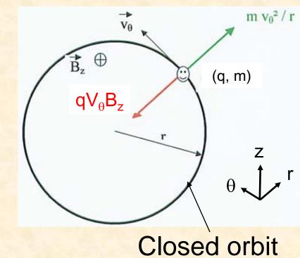
Conventional cyclotrons means *non relativistic* cyclotrons low energy  $\Rightarrow \gamma \sim 1 \Rightarrow m / m_0 \sim 1$
