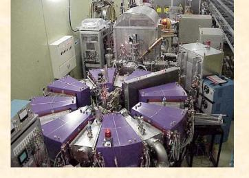
1 MeV proton beam 2.5 m diameter experiment at the Japanese KEK laboratory has demonstrated fixed-field proton acceleration. 150 MeV FFAG accelerator complex in Research Reactor Institute, Kyoto University (KURRI). ADS experiments using this accelerator has been started in March of 2009.
