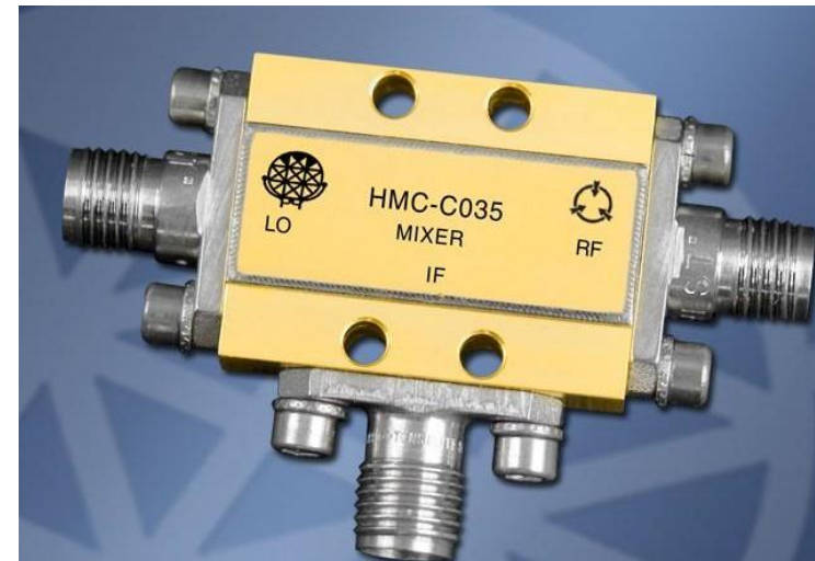
A typical coaxial mixer (SMA connector)
