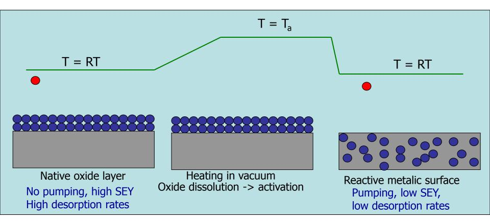
NEGs pump most of the gas except rare gases and methane at room temperature
