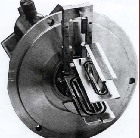
IBA Cyclone 18/9, Cyclotron in Geneva 9 MeV Deuteron beam spot on the Havar Window foil of the Ne(F<sub>2</sub>) [<sup>18</sup>F]F<sub>2</sub> target
