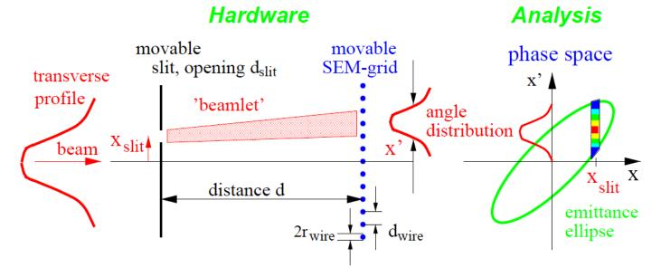
For pulsed LINACs: Only one measurement each pulse  $\rightarrow$  long measuring time required.
