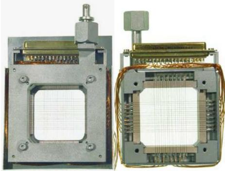
Each wire is equipped with one I/U converter different ranges settings by  $R_i$  $\rightarrow$  very large dynamic range up to 10<sup>6</sup>.
