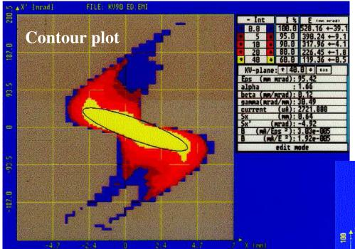
Low energy ion beam: → well suited for emittance showing space-charge effects or aberrations. ➢ different evaluation and plots possible
