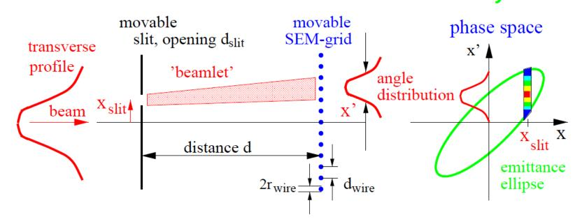
*Slit*: position P(x) with typical width: 0.1 to 0.5 mm *Distance:* 10 cm to 1 m (depending on beam velocity) *SEM-Grid:* angle distribution P(x')
