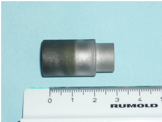
Object found inside the RF wave guide. It was a device used in the brazing oven
