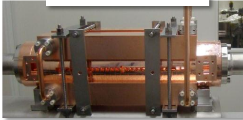
TD24 accelerating structure
