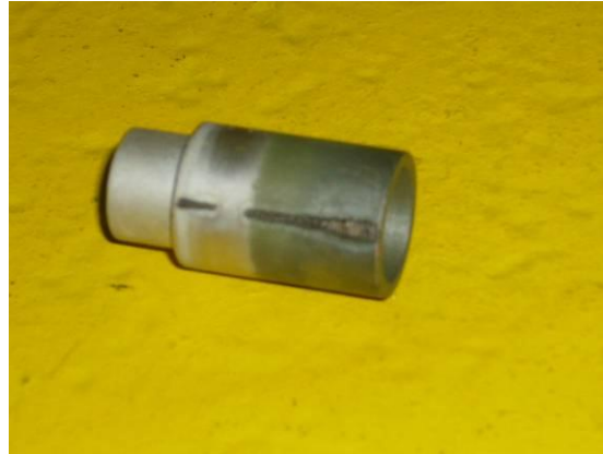
Object found inside the RF wave guide. It was a device used in the brazing oven
