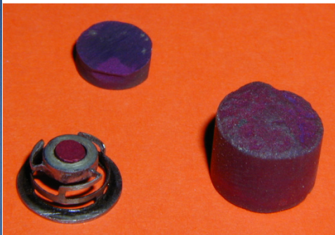
cathodes damaged by sputtering (see later)
