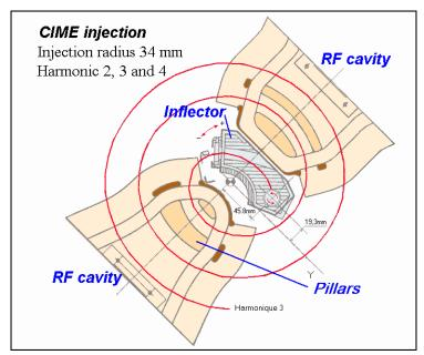
If  $r_0$  is the first and unique radius of curvature of the orbit at the exit of the inflector, find a relation linking the mean magnetic field  $B_0$ , the RF frequency  $F_{RF}$ , h the harmonic number and the ion source plateform voltage  $V_{inj}$ :  $\frac{1}{\pi \cdot r^2_0} = \frac{F_{RF} B_0}{h V_{ij}}$
