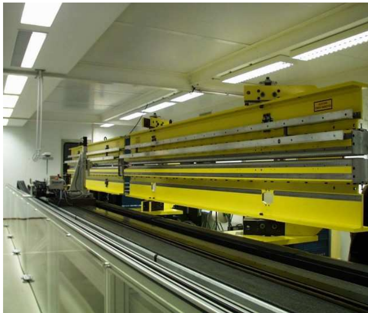
Undulator of the SASE-FEL (DESY)
