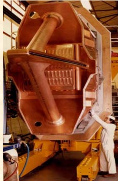
Copper skinned inner conductors with 'Dee' (inner electrode)
