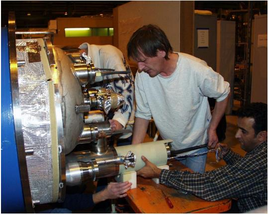
Installing the cold diode package on the end of an LHC dipole
