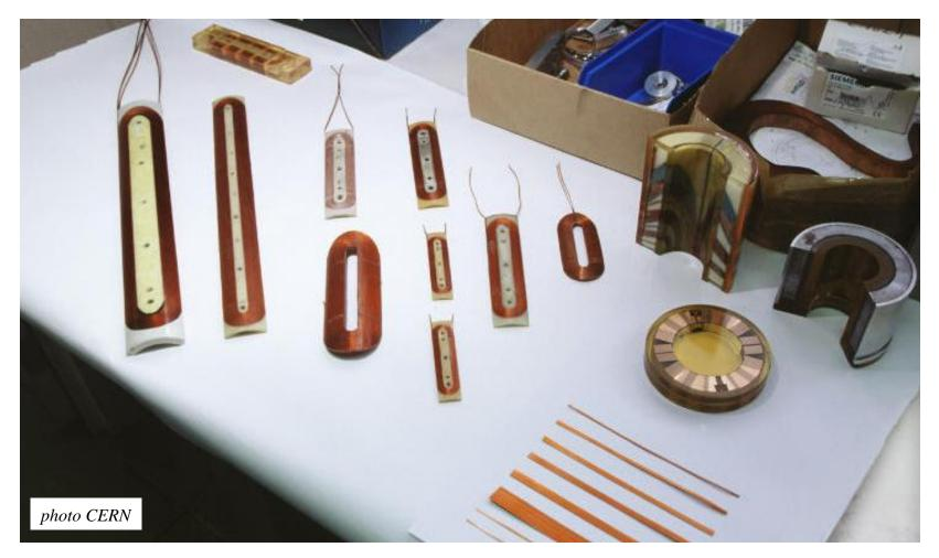
On a smaller scale, but in great number and variety, many different types of superconducting correction coils are needed at a large accelerator
