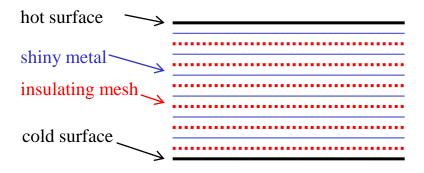
Because radiated power goes as  $\theta^4$  you can reduce it by subdividing the gap between hot and cold surface using alternating layers of shiny metal foil or aluminized Mylar and insulating mesh.
