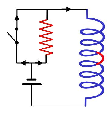
Note: circuit breaker must be able to open at full current against a voltage  $V = I.R_p$  (expensive)
