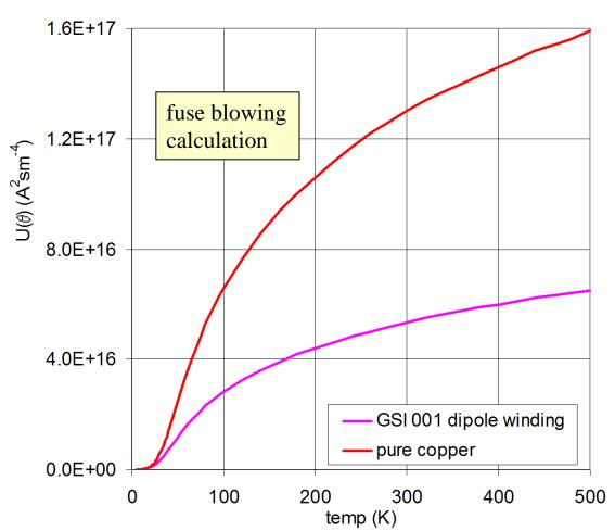
household fuse blows at 15A, area =  $0.15 mm^2$  J =  $100 Amm^{-2}$  NbTi in 5T  $J_c = 2500 Amm^{-2}$
