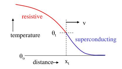
$$\frac{\partial}{\partial x} \left( kA \frac{\partial \theta}{\partial x} \right) - \gamma CA \frac{\partial \theta}{\partial t} - hP(\theta - \theta_0) + J^2 \rho A = 0$$
