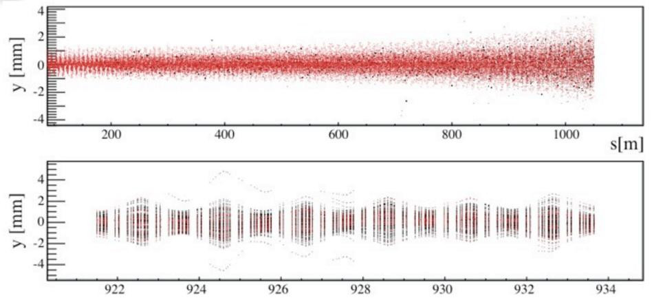
Vertical beam position along a complete CLIC decelerator + zoom towards end Halo particles are shown in **black**, **beam** (**core**) **particles in red**
