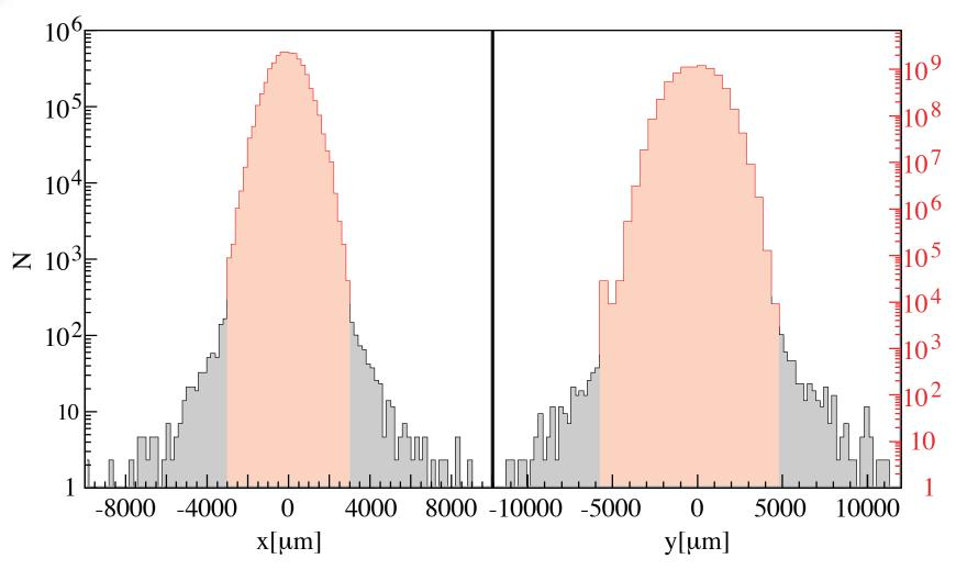
Transverse Beam profiles at the exit of the CLIC decelerator PLACET + HTGEN simulation
