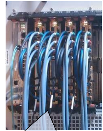
VME Crate with 4 BPM electronics (see FEL2010, WEPB15).
