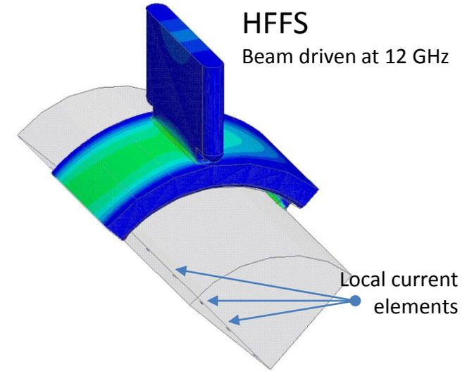
➤ Big cavity volume results in the rather dense dipole modes spectrum. Special care should be taken (the cavity shape, damping?) to avoid resonant conditions at harmonics of 12 GHz.
