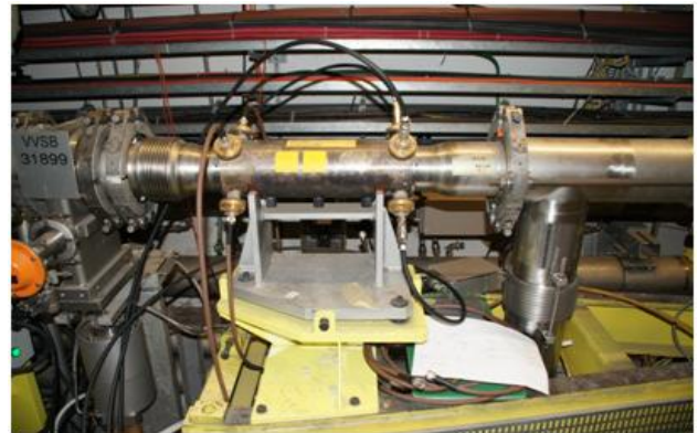
Figure 12: Picture of the pick-up installed in the SPS ring.
