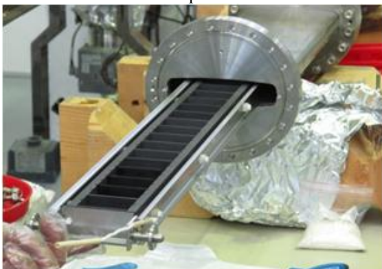
Figure 2: Picture of the hollow-cathode being inserted in the MBA dipole magnet beampipe profile.
