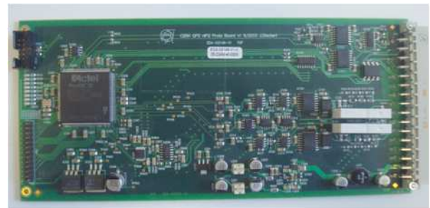
Figure 1: Radiation tolerant quench detection board for insertion region magnets and inner triplets
