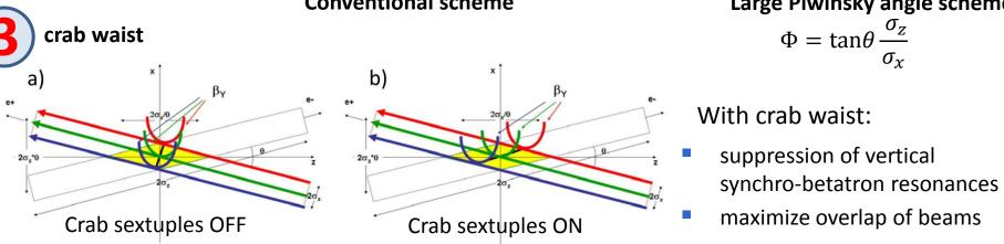
Collision scheme with large Piwinsky angle + crab waist successfully tested at DAFNE in 2009 (3x luminosity increase with CW ON). New tests ongoing at DAFNE with KLOE-2 installed (0.5 T solenoidal magnetic field ON)
