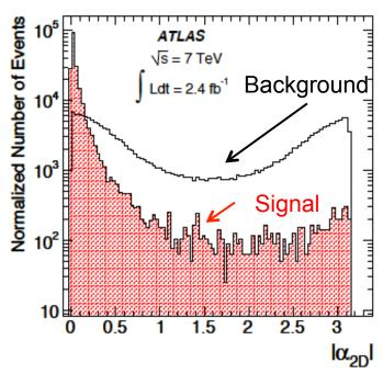
$\alpha_{2D}$  = angle between  $\Delta x$  projection in transverse plane and B transverse momentum
