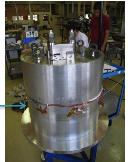
Coil pack and Iron yoke mounted in the instrumented Al2219 T851 shell
