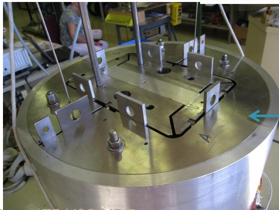
Coil pack and Iron yoke mounted in the instrumented Al2219 T851 shell
