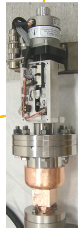
Movable RF short circuit (to tune the resonant length)
