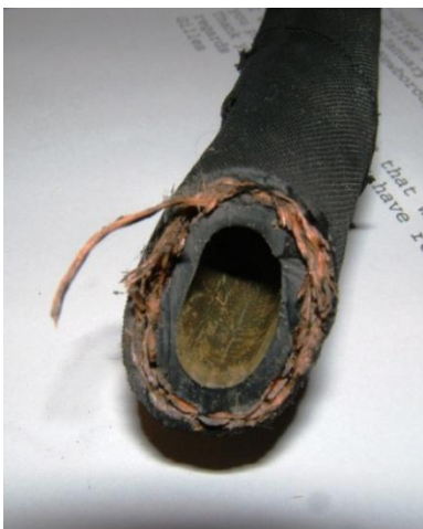
Delaminated cooling hose
