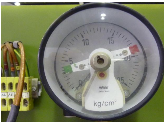
Manometer with gold tip contacts corroding due to water pressure oscillations
