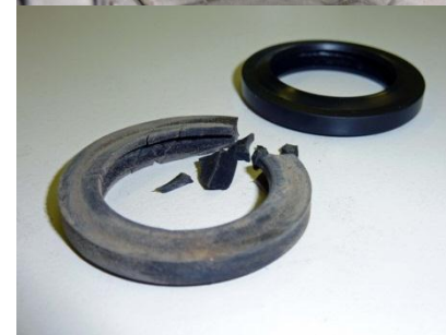
Quick connector gaskets degraded by irradiation
