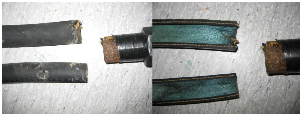
Burst cooling hose
