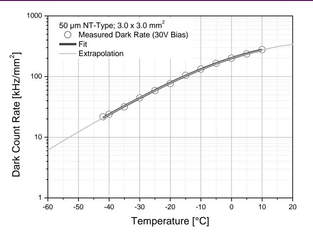
The dark rate is scaling with the carrier density in silicon
