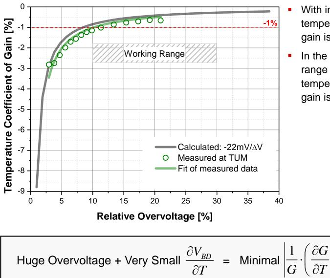
With increasing overvoltage the temperature coefficient of the gain is decreasing drastically
