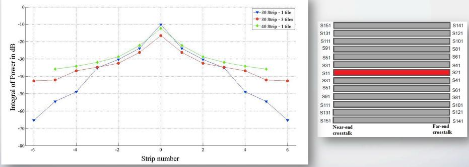
Measurement of the crosstalk as a function of the strip number on the anodes
