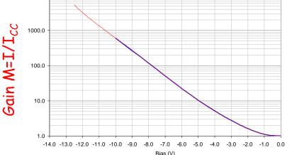
MWIR HgCdTe e-APD cut-off wavelength  $\lambda_c$ =5.3 µm T=80K
