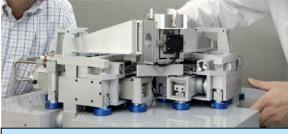
Guide ways for NANO-CMM Accuracy: 0.2 µm straightness over 300 mm
