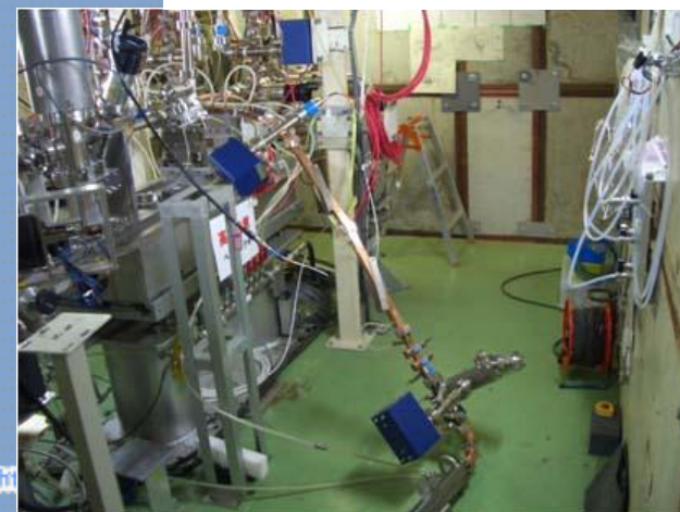
Nextef collapse due to non-fixed load
