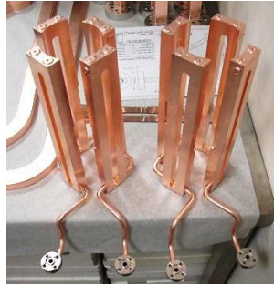
Assembly of cooling circuits
