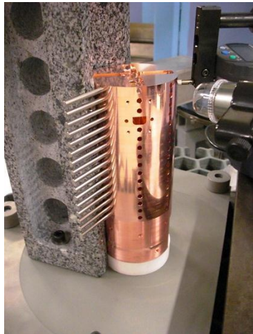
Assembly of disks in the furnace
