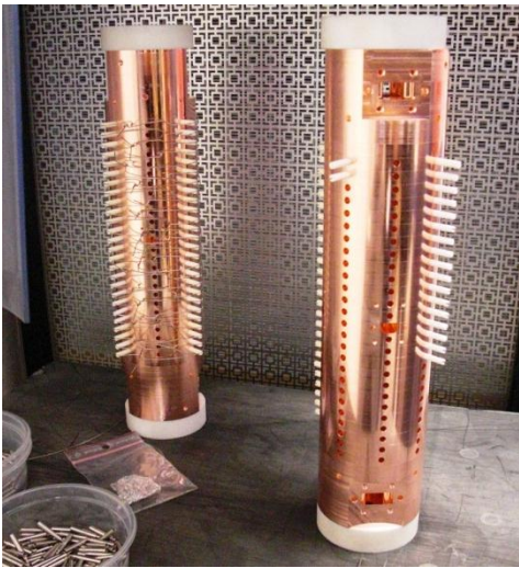
Assembly of tuning studs
