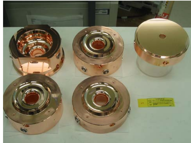
An rf-gun cavity and pipes were brazed in Hydrogen furnace.
