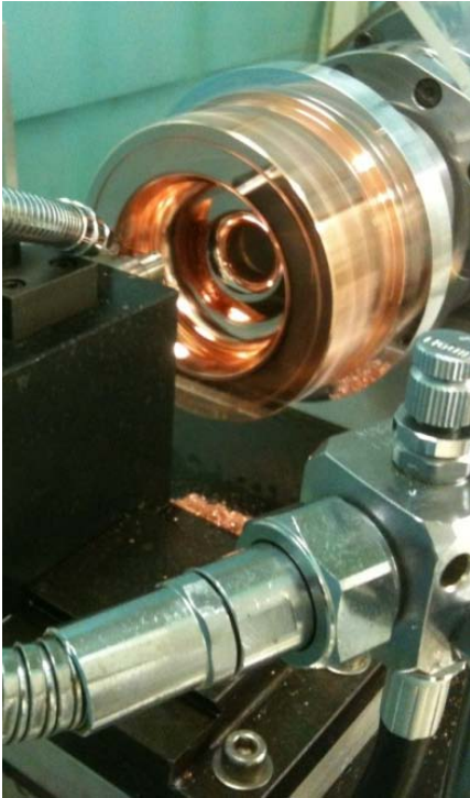
Cutting by Diamond turning
