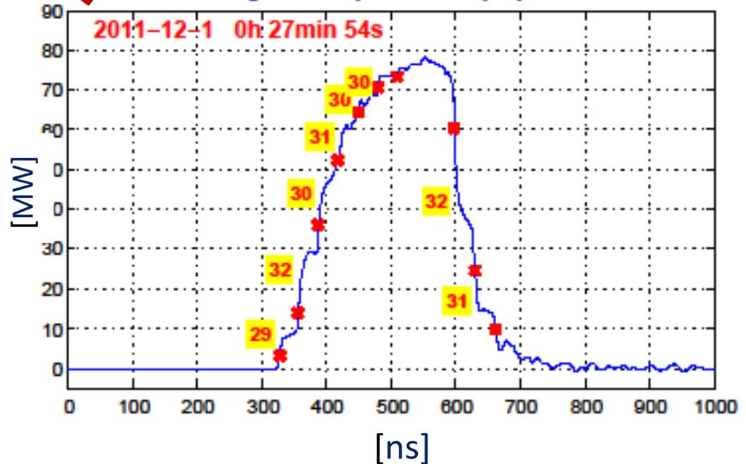
Average input signal and steps detection showing the recirculation loop delay of 31 ns
