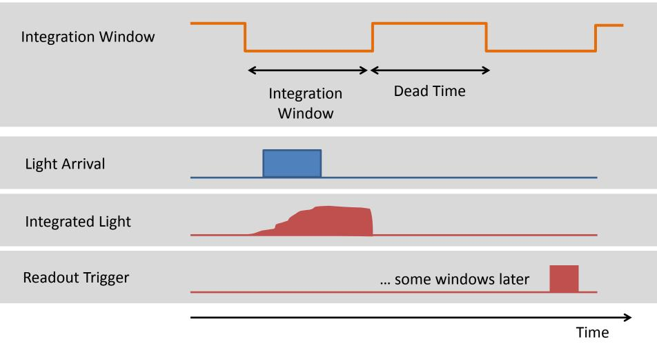
• The tracker needs to be synchronised to incoming particles so that the alive window is in the right place.
