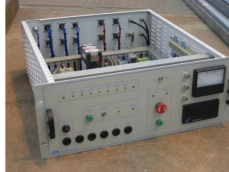
HV PSU Control Unit
