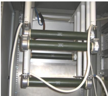
38 kV PSU – resistor bank
