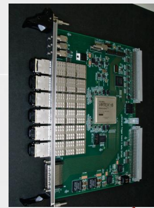
UT3-β shown in Feb. 2010 24 RocketIO (GTX, 6.25Gbps) FPGA: Xilinx XC6VLX240T
