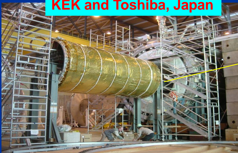
Central Solenoid during integration in the common cryostat of the Liquid Argon Barrel detector at hall 180
