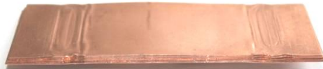
EMPT welding of foil stacks: 10 x 250 µm Cu
