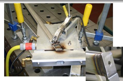
Parts are welded in custom made cooled aluminum block under inert gas flow on both sides of the weld for UHV compatibility
