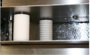
Insets for ultrasonic cleaning of wires
