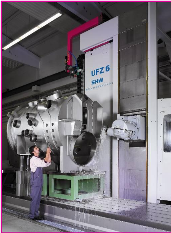
5-axis CNC machining center for large components.
