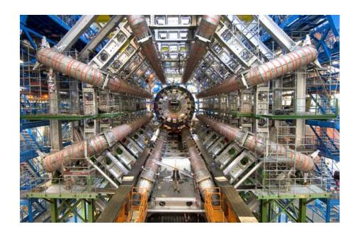
To sample and record the debris from up to 600 million proton collisions per second, scientists are building gargantuan devices that measure particles with micron precision.
