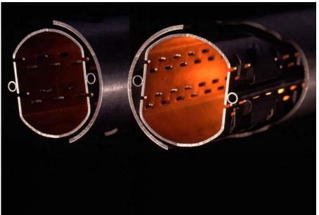
To accelerate protons to almost the speed of light requires a vacuum as empty as interplanetary space. There is 10 times more atmosphere on the moon than there will be in the LHC.
