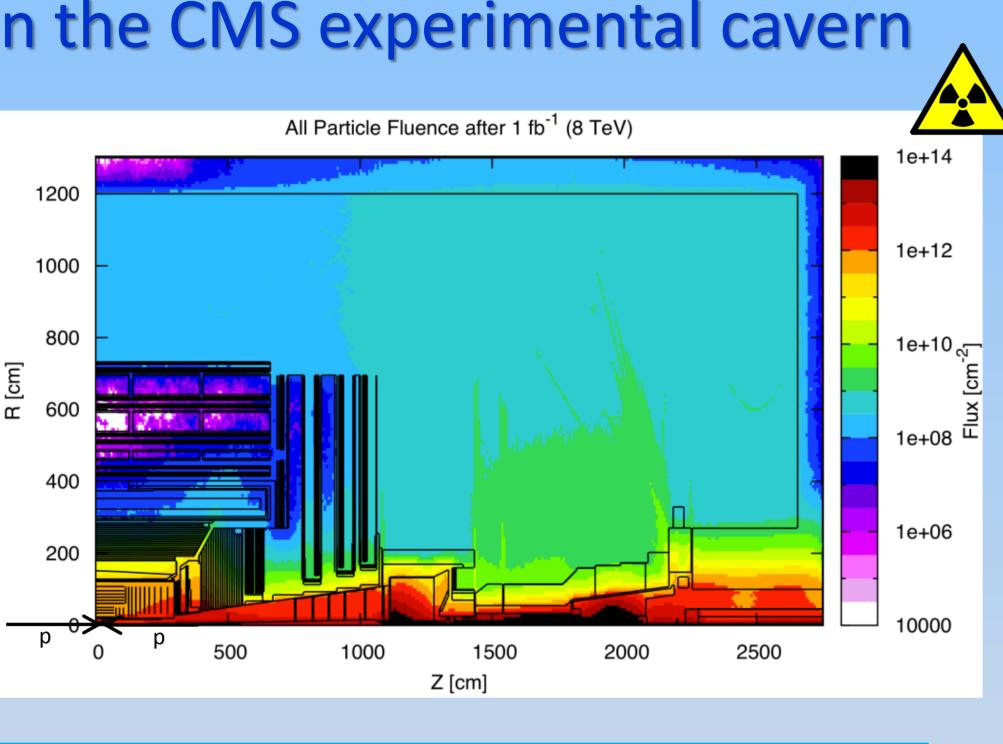
Electronics in the experiment are exposed to radiation from proton collisions
