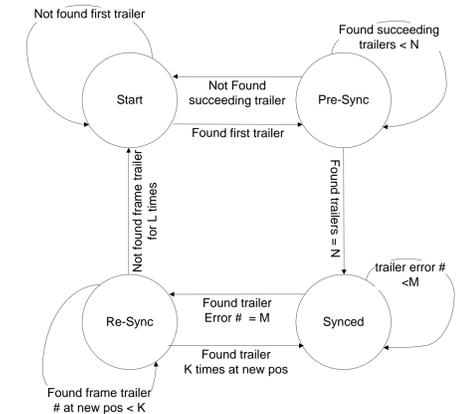
The state machine of frame synchronization process
