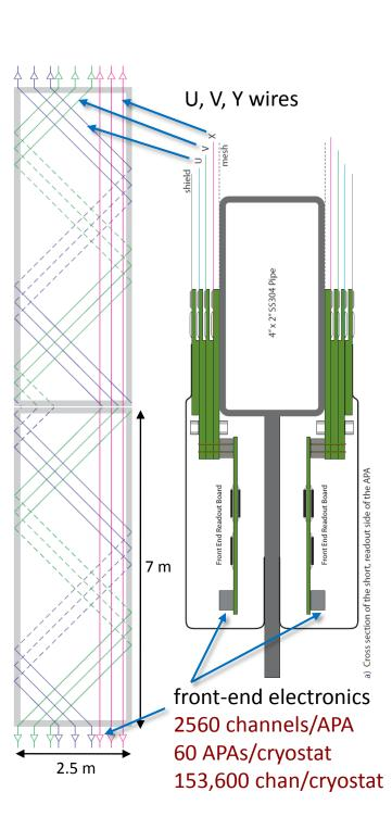
all sense wires and readout electronics. They are standardized manufactured assemblies, can be tested in LN2, stored and transported in shipping containers.
