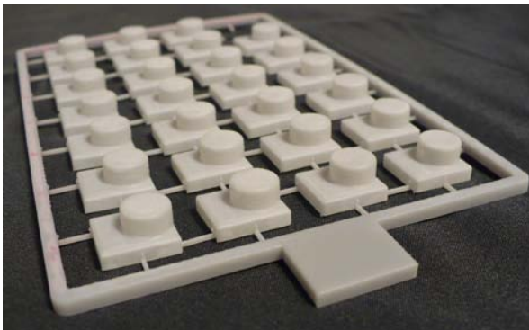
Protopes made with rapid prototyping
