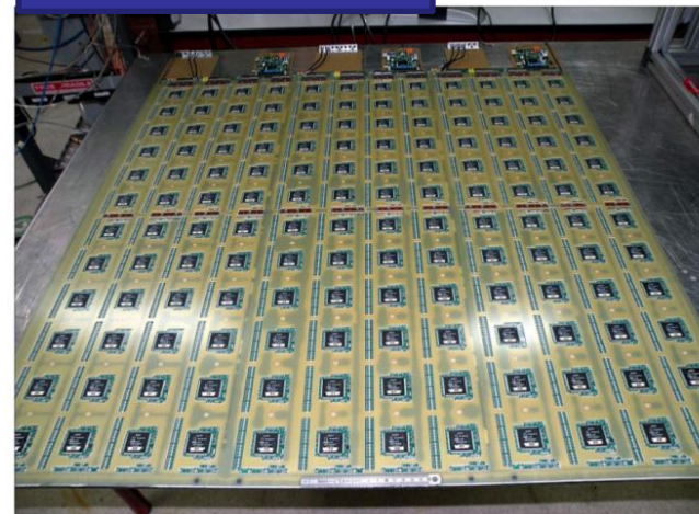
1m 2 equipped with 144 MICROROC
