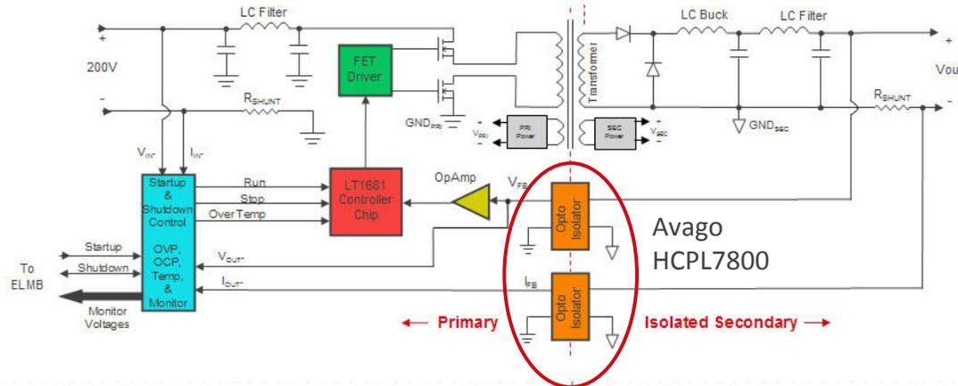
**Opto-Isolator Circuit Schematic**
