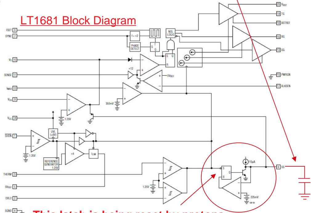
**This latch is being reset by protons**
