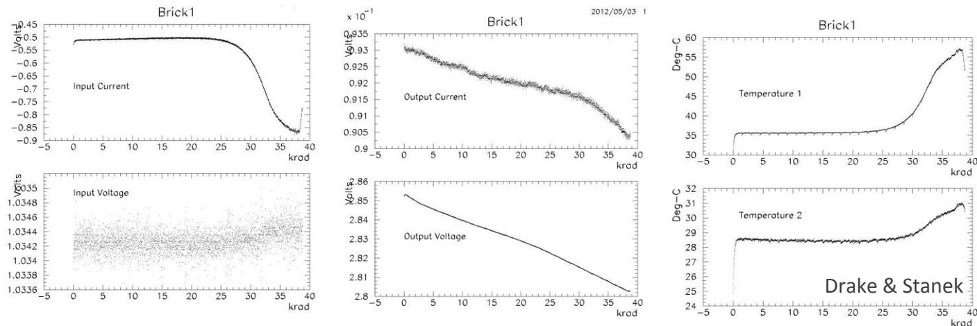
⇒ **Retest to look for opto-isolator failure at high dose**
