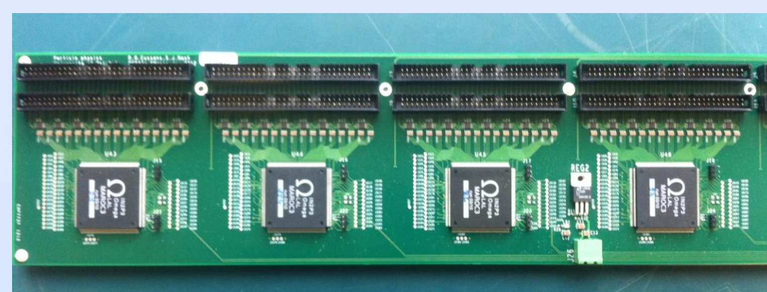
A section of the readout board, which uses five MAROC3 chips read-out by a Xilinx xc6slx16 FPGA
