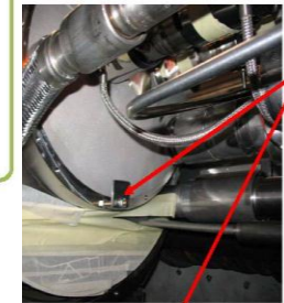
Half yoke samples, fixed with stainless steel threaded rod (M10x100mm), 3 washers and 3 nuts.
