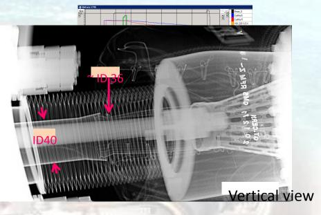
NC found during Xmas shut down: **RF fingers overlap of ~ 6 mm inside RF insert** exactly where the pressure increase had been observed
